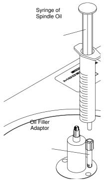
7. Remove the syringe from its packing and insert the tip into the Oil Filler Adaptor, which will be found already fitted to near the spindle. (as illustration left).
